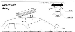
of SNm. Drill 4 holes 9mm diameter at required fixing centres shown.
